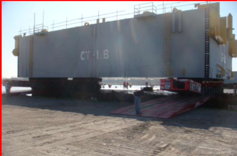
Th second barge makes its way up the ramps onto the deck barge.
